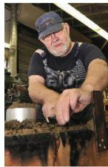
Harold Chandler, a worker from the Fleet Maintenance Facility's (FMF) foundry, works on the sand mould for the Naval Centennial Bell.
